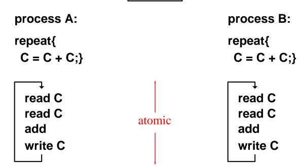
Theorem? For every positive integer n there is an interleaving of A and B steps that produces  $\mathsf{C} = n$ .
