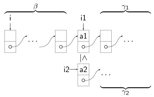
$\begin{array}{l} \mbox{if } \mbox{n1} = 1 \mbox{ then } [\mbox{i1} + 1] := \mbox{i2} \mbox{; goto out else} \\ \mbox{n1} := \mbox{n1} - 1; \end{array}$
